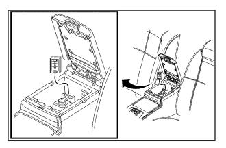
Place the new, unrecognized transmitter into the transmitter pocket with the transmitter buttons facing the front of the vehicle. The transmitter pocket is inside the center console storage area located between the driver and front passenger seats.
